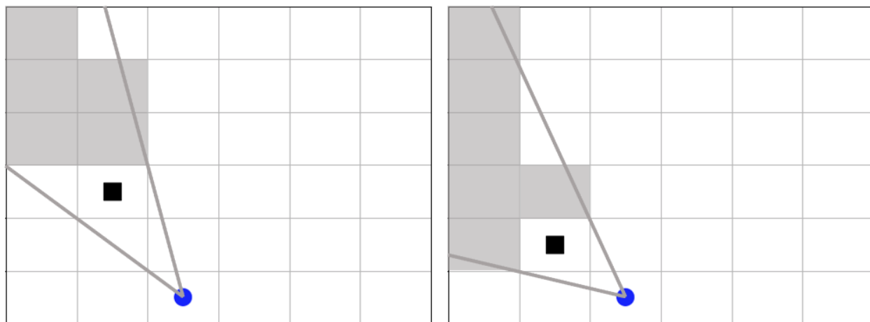
Fig. 4: The black agent is a wall agent that masks part of the grid from the blue agent. Cells whose centers fall between the lines are masked. Centers that fall directly on the line or outside of the lines are not masked. Two setups are shown to demonstrate how the masking may change based on the agents' positions.
